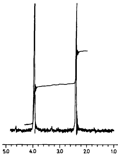
Figure 4: NMR signals used for quantitation of 2-acetoxy-4-trifluoromethylbenzoic acid in the presence of vanillin ( \delta 4.0), as reference compound, in chloroform.
